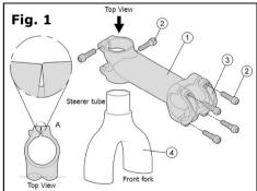
Important Note: Carbon steerer tubes must extend through the Whyte stem completely for proper clamping pressure. It is necessary to have 2mm minimum of steerer tube extended above the stem together with the use of a minimum 5mm headset spacer between the Whyte stem and headset cap for ALL carbon steerer tube forks. See figure 2. Ensure that the steerer tube is clean and free of burrs or chips before installing the Whyte stem onto steerer tube.
