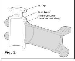
Tighten the stem fixing bolts ② by alternating between bolts 1/4 turn at a time so both bolts reach proper torque simultaneously. **DO NOT** go above maximum torque rating displayed on the stem. If two fixing bolts go over the maximum torque, the stem clamps may touch slightly (as shown in view A, figure 1). This is **NOT PERMISSIBLE** since it will compromise the strength of the joint, reducing it's service life and may cause injury or death to persons or damage to property as a result.
